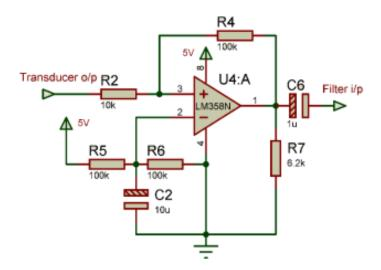
It is feasible to achieve a maximum output voltage of 200 mV is the preamplifier. Therefore, to increase the power, a voltage boost of 20 dB is necessary. To construct this pre-amplifier, researchers followed the standard application circuit described in the LM358 datasheet, making only the most fundamental adjustments. Figure 2 shows the pin diagram of the LM358 and the preamplifier circuit in detail.
