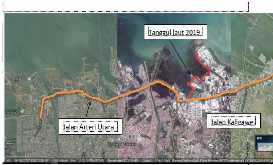
Figure 1. The sea embankment completed in 2019 and the North Arterial Road also function as a tidal barrier (Heryoso Setiyono, 2023)
